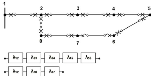
Figure 2. EDN with circuit breakers and its corresponding reliability block diagrams for peripheral customers (6 and 7)
