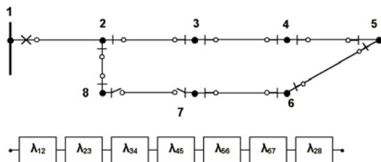
Figure 1. EDN with switchgears and/or switch disconnectors and its corresponding reliability block diagram
