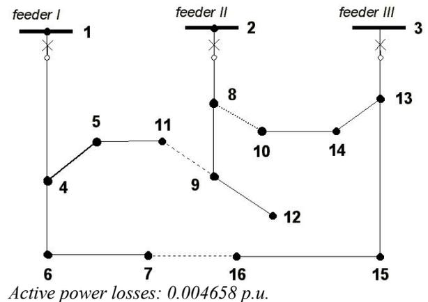
Fig. 4. Test 16 bus network – optimal configuration
