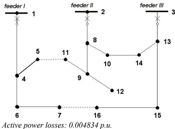
Fig. 3. Test 16 bus network – configuration obtained applying branch-exchange method
